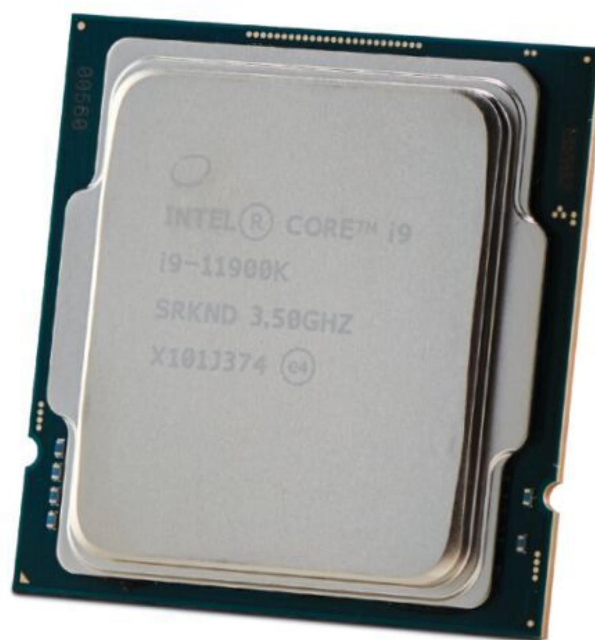
Meanwhile, the i9-11900K has gone back to just eight cores, but still manages to take up 276.4mm 2 of space.
