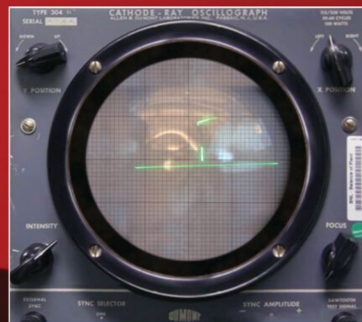
Tennis for Two on an oscilloscope and played with two custom aluminum controllers.
