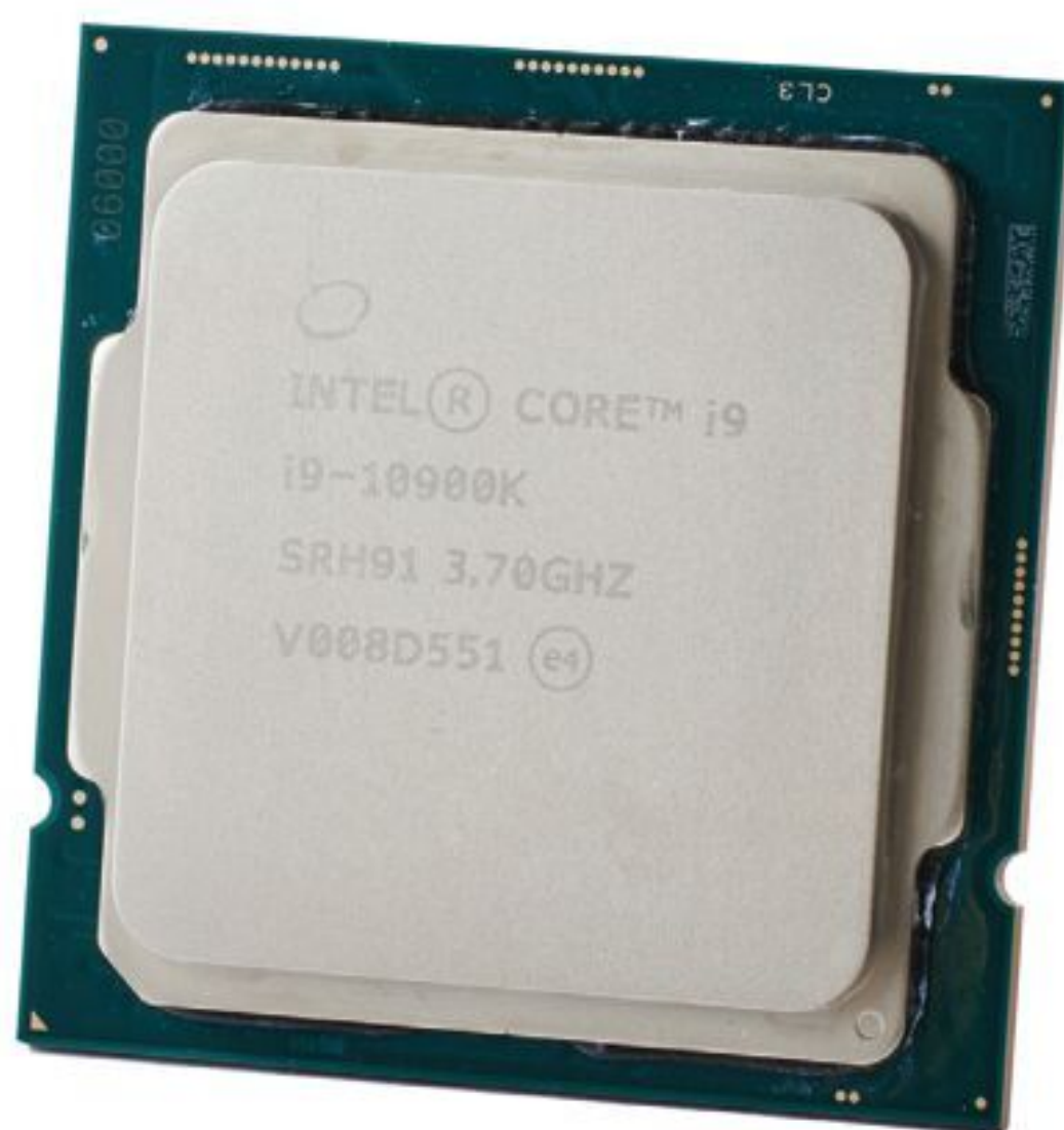
Measuring a relatively dainty 206.1mm 2 , the Comet Lake Core i9-10900K squeezed in 10 CPU cores alongside 24 GPU EUs.
